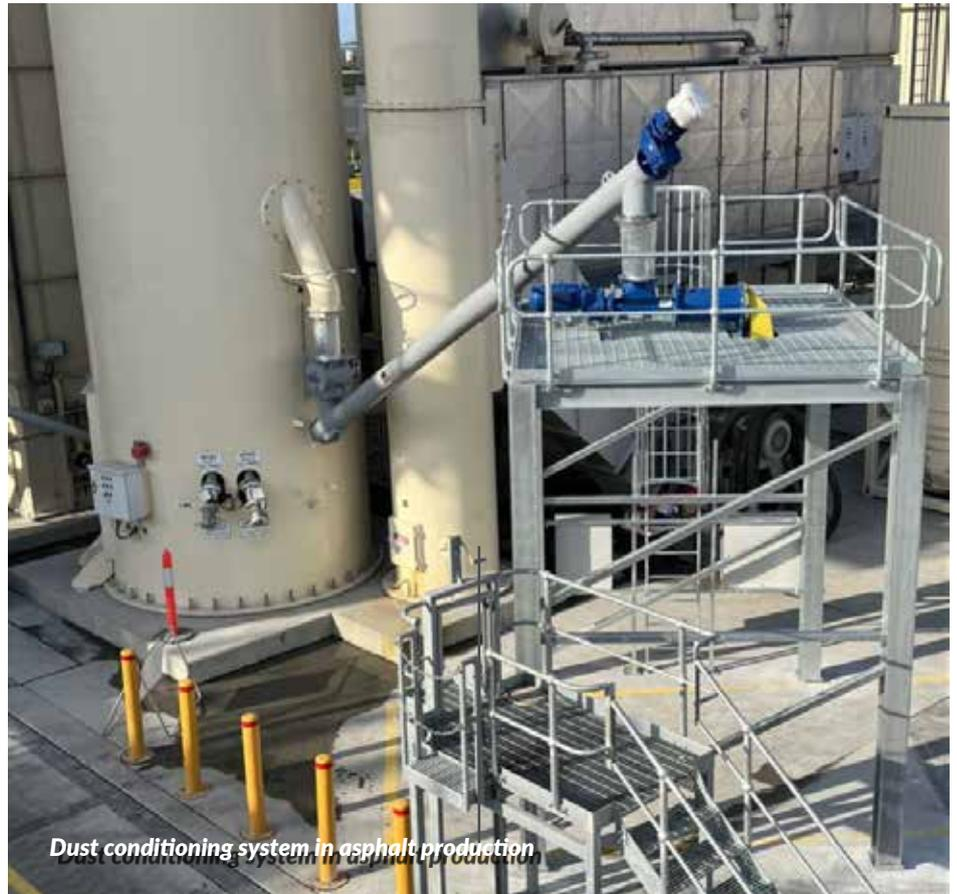
A TOREX® Drop-through Rotary Valve as a fundamental component ensures efficient and precise material flow, facilitating the overall functionality of the system.
